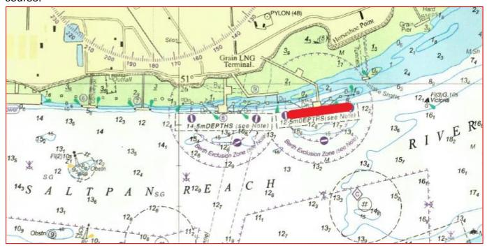
All vessels passing Grain LNG Jetty 10 should navigate with caution, observe the LNG Jetty exclusion zone at all times and reduce speed and wash accordingly.
