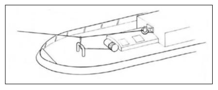
It will be appreciated from the illustration above that a gog rope can limit how far the tug can turn at the end of the towline. In certain circumstances, improper use of a gog rope can severely restrict a tug's manoeuvrability and effectiveness. Therefore, tug operators using a tug to tow conventionally should provide specific training and instruction to the tug master regarding when a gog rope must be used, and on the effectiveness and limitations of using a gog rope.
